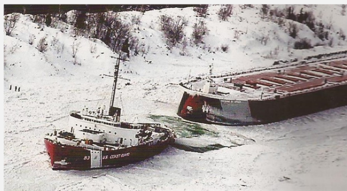
The Mackinaw WAGB-83 at full throttle while attempting to use "prop wash" to free the Speer . Notice the people observing from the shore. The effort lifted the bow of the Mackinaw right out of the water. Crew commented on the difficulty moving forward through the ship on her rising decks.
